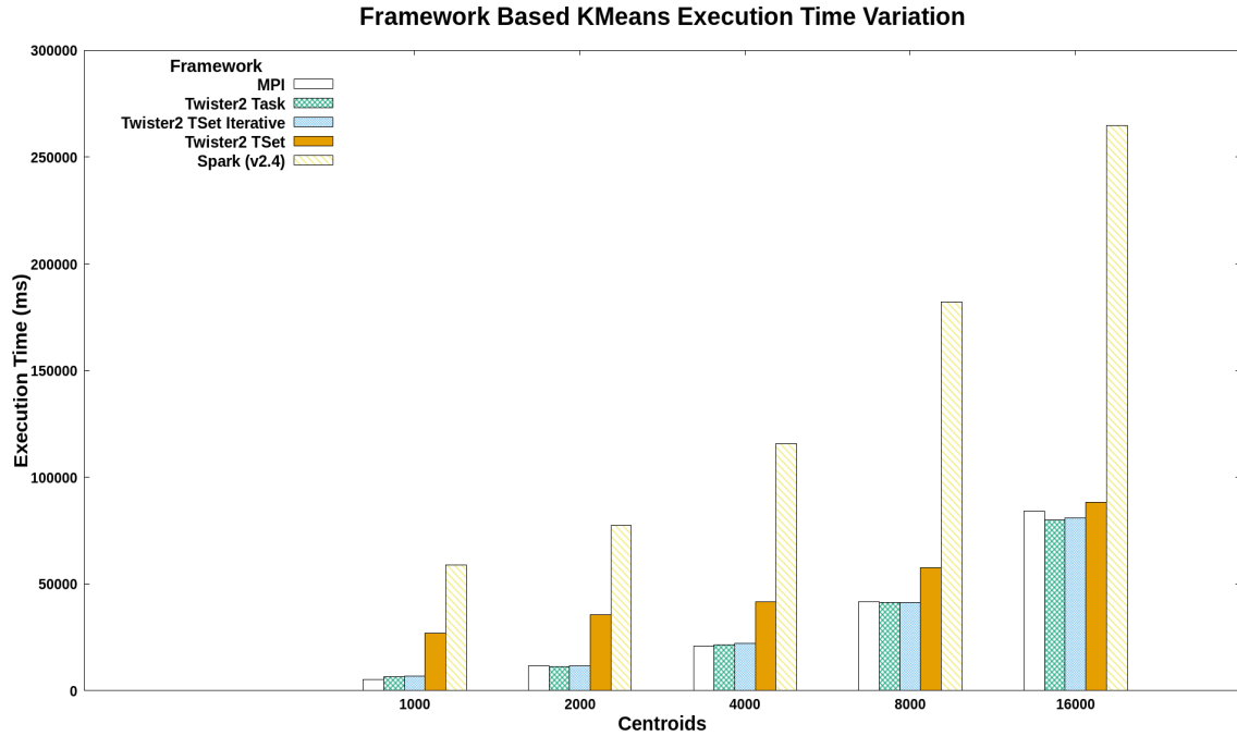
FIGURE 5 K-Means job execution time on 16 nodes with varying centers, 2 million data points with 128-way parallelism for 100 iterations.
